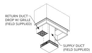
**RUSKIN'S SOD SERIES** supply diffuser systems are designed to provide an air distribution system with the benefit of having directional air control. The system is ideal for open ceiling applications that need single point supply air with control over where the air is distributed.
