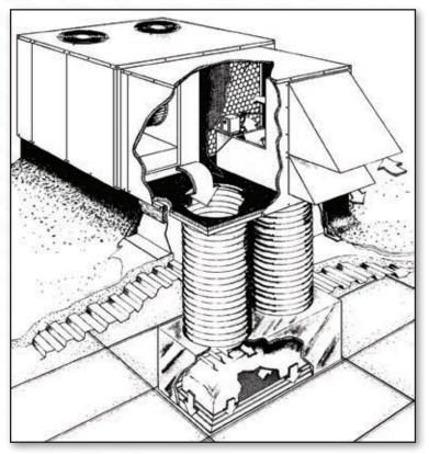
This CAD rendering demonstrates the supply and return air paths from the rooftop AC equipment into the concentric diffuser. Concentrics make the installation of the single diffuser easier by reducing the complexity of ductwork and transitioning within the concentric plenum.
