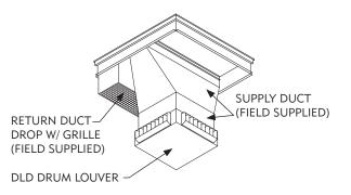
**RUSKIN'S DLD SERIES** supply diffuser systems are designed to provide an air distribution system with the benefit of having directional air control. The system is ideal for open ceiling applications that need single point supply air with long throws. The Drum Louver allows you to "spot" the air where you need it the most.
