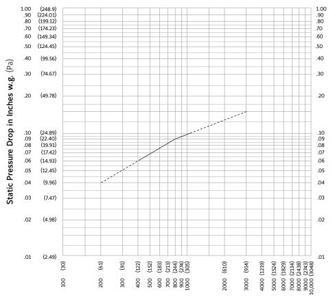
Air Velocity in feet (meters) per minute through Free Area Maximum recommended free area exhaust velocity through louver: 1,500 fpm (457 m/min).
