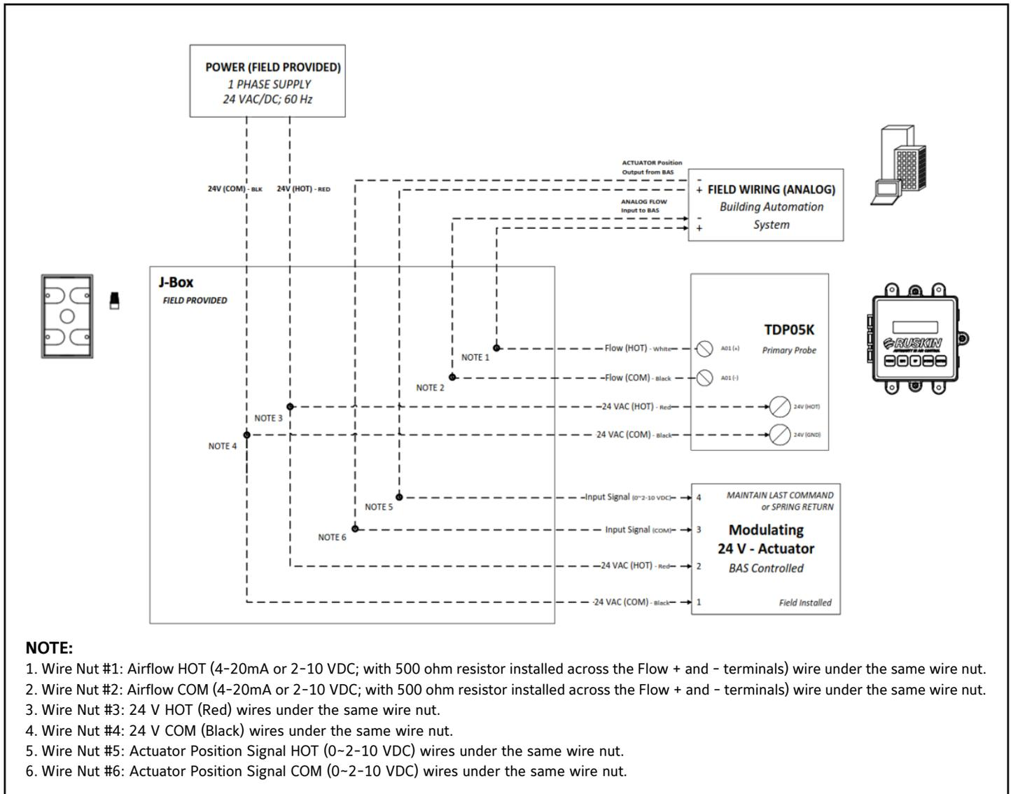
FIGURE 16: AIQ-TD-xx Analog Field Wiring
