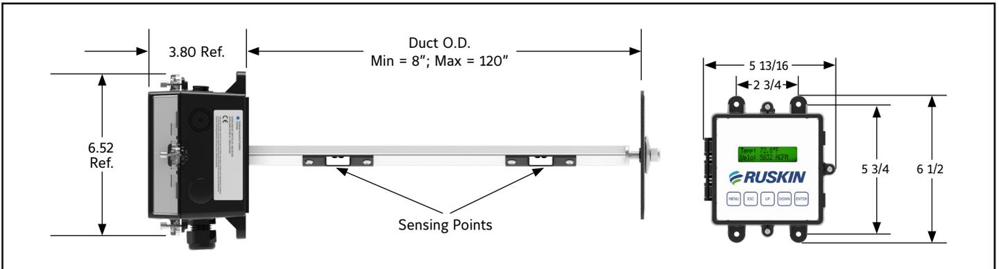
FIGURE 8: TDP05K Airflow & Temperature Measuring Probe and Face of Primary Monitor Box (User Interface)
