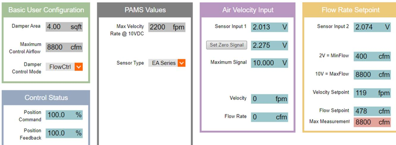
FIGURE 22: Configurations GUI (VA\*B24-BAC Air Measurement Actuator)
