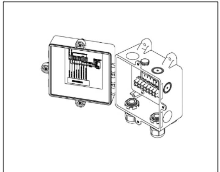
FIGURE 4: Factory-Mounted Junction Box. Includes Wiring Diagram on Internal side of Lid Cover.
