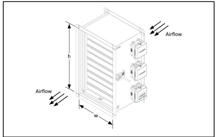
FIGURE 11: RIGHT HAND Mount Airflow enters through the TDP05K probes and exits through the control damper.
