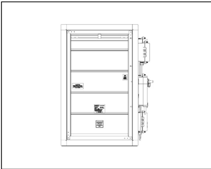
FIGURE 3: Control Damper mounted within Sleeve. Shown with Optional Rear Flange and viewing from Downstream of the Installation
