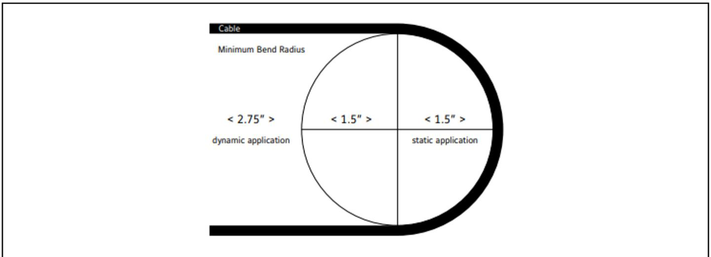
FIGURE 16: Wire - Minimum Bend Radius
