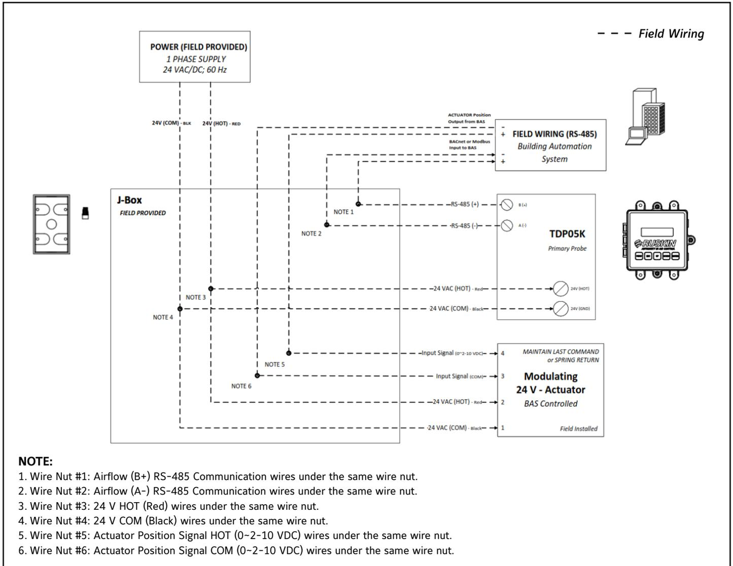
**FIGURE 18: AIQ-TD-xx BACnet or Modbus Field Wiring**
