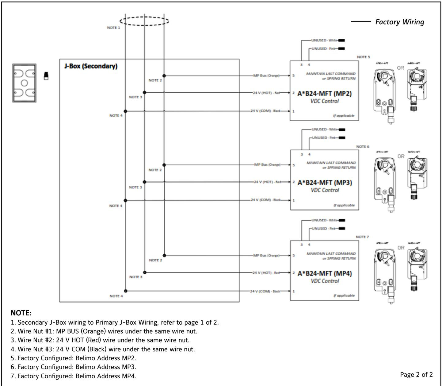
**FIGURE 17b: AIQ-TD-xxC Analog Field Wiring**
