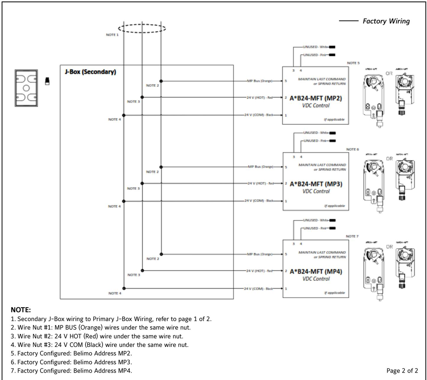
FIGURE 19b: AIQ-TD-xxC BACnet or Modbus Field Wiring
