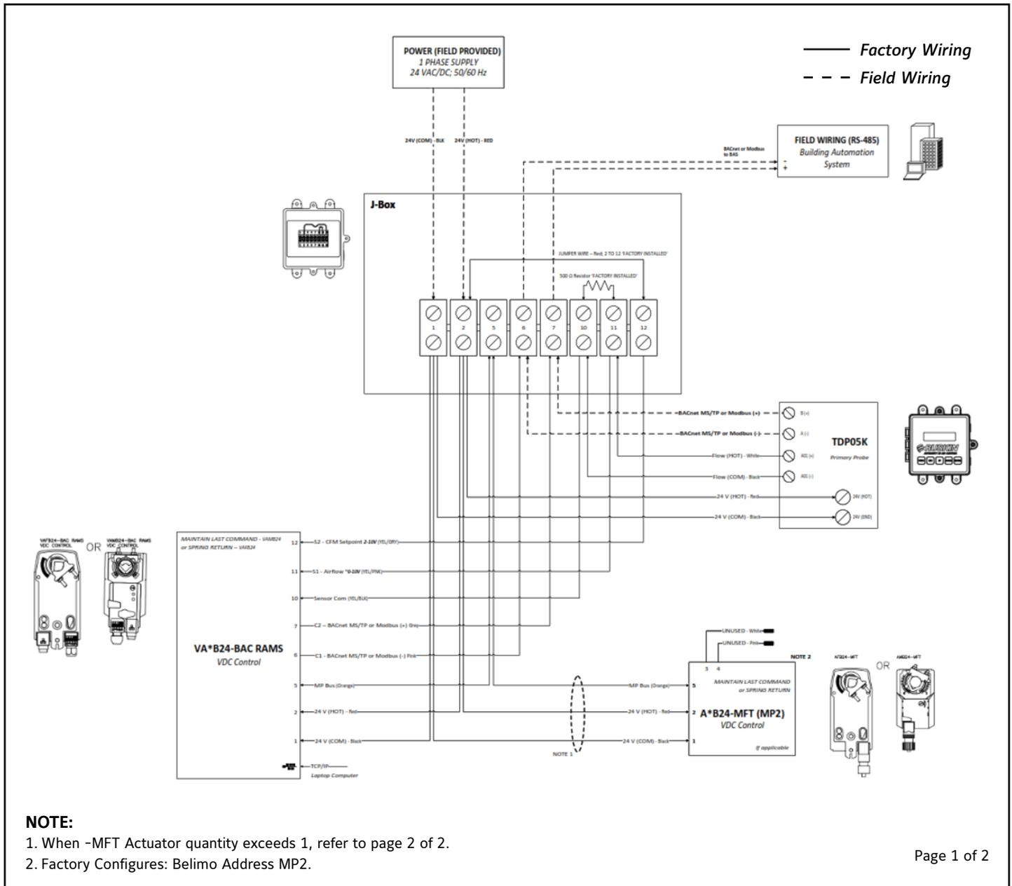
FIGURE 19a: AIQ-TD-xxC BACnet or Modbus Field Wiring
