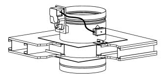
A **square** opening in wood or metal stud "tunnel" corridor ceilings shall be a minimum of 1" (25) and a maximum of  $2^{1/2}$ " (64) larger than the damper diameter.
