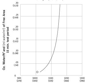
Free Area Velocity in feet and (meters) per minute Standard air .075 lb/ft³ (1.2 kg/m³)
