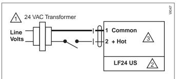
Provide overload protection and disconnect as required.
