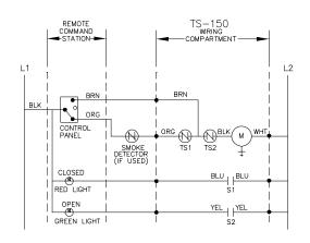
M - ELECTRIC ACTUATOR OR EP-SWITCH
