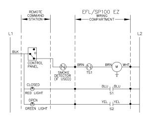
M - ELECTRIC ACTUATOR OR EP-SWITCH
