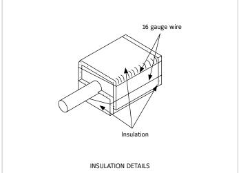
NOTE: Installation without the insulation does not provide protection of the opening. Insulation must cover surfaces as shown.
