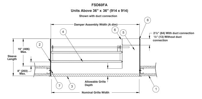
FSD60FA dampers larger than 36" x 36" (914 x 914) are installed with grille on opposite side of damper from jackshaft.
